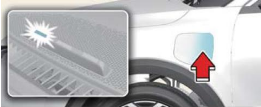
Operation of charging indicator lamp
