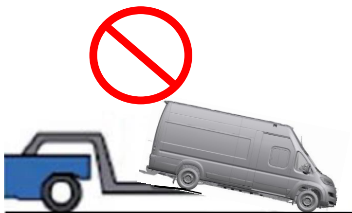
DO NOT TOW WITH WHEELS ON THE GROUND
