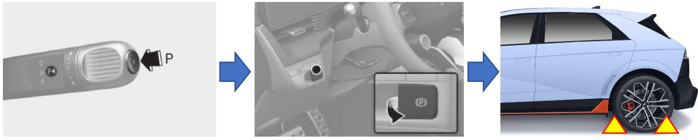
Put the vehicle in P (Park) position by pressing the 'P' button on the rotary shifter
